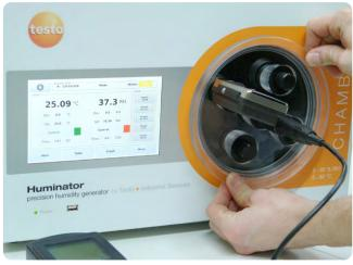
The Huminator II is designed to carry out fast and precise humidity calibrations. In laboratory use, where fast processing times and continuous operation are of crucial importance, the Huminator is characterized by its outstanding performance and its reliability.
